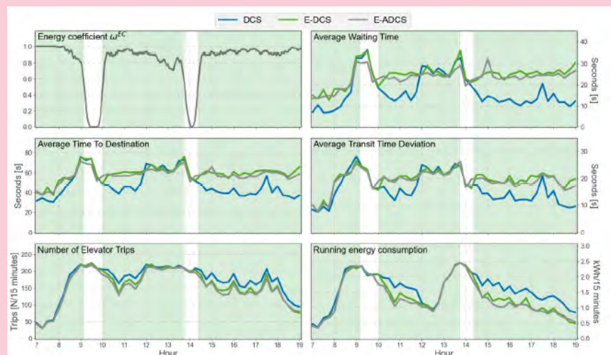
Figure 2: Several KPIs plotted as a function of time for elevator group L4, with the DCSs under daily multi-tenant office demand.
