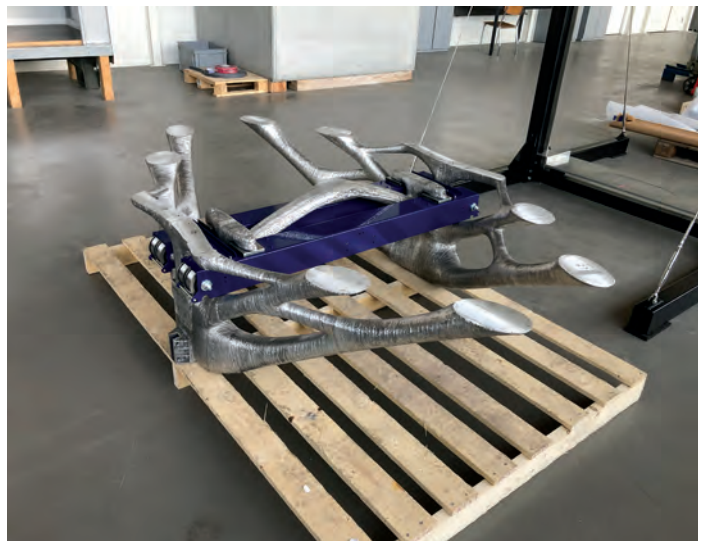
Floor structure ready to be mounted; courtesy of MX3D
