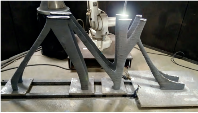
Welding robot during the “printing” process of car parts; courtesy of MX3D
