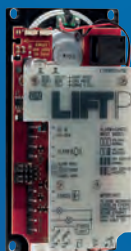
Lift IP VoIP elevator phone
