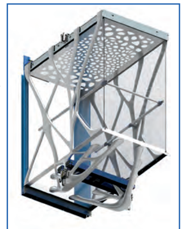
3D CAD drawing of printed car; courtesy of Schindler
