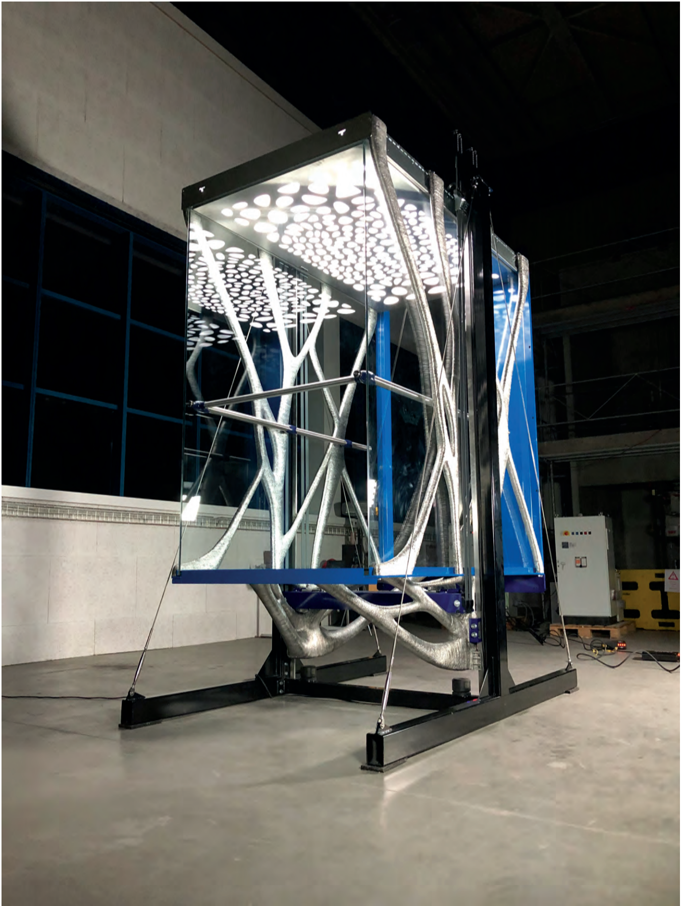
Assembled elevator car with standard car roof; courtesy of Schindler
